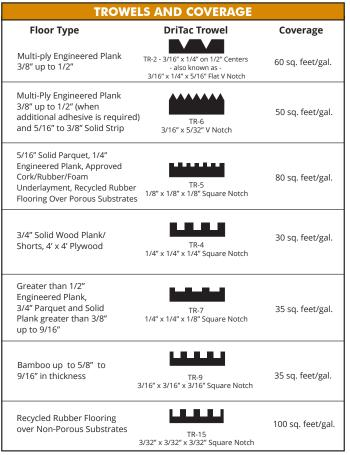
Trowels diagrams are not to scale. Use DriTac 7300 adhesive with a properly notched trowel. All square footage rates are estimated. Rates will vary based on substrate condition and the angle the trowel is held to the subfloor. Failure to properly flatten the subfloor may result in hollow spots. DriTac warranties do not cover problems caused by improper use of installation products. Follow flooring manufacturer's written installations instructions.
